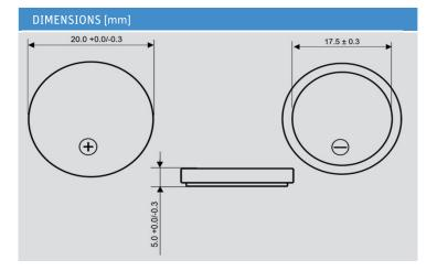
Note: Capacity 300mAh is obtained at standard cc load to 2.0V at 23°C.
