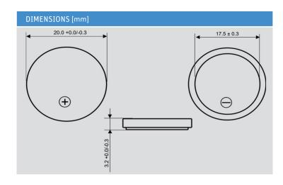
Note: Capacity 200mAh is obtained at standard cc load to 2.0V at 23  $^{\circ}\text{C}.$
